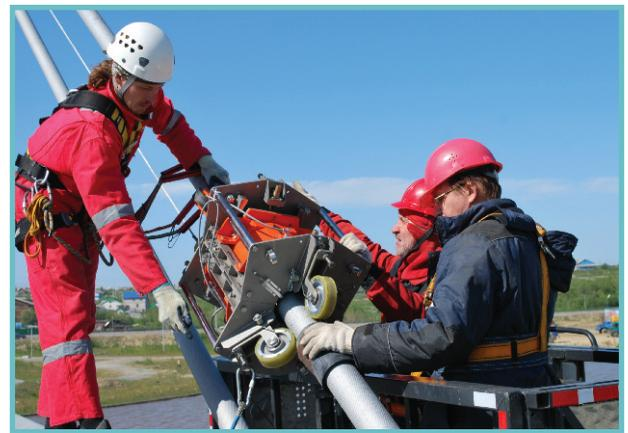
Figure 2. Inspection of a 95 mm (3.8 in.) stay bridge rope with a magnetic flux leakage testing instrument with roller system.
