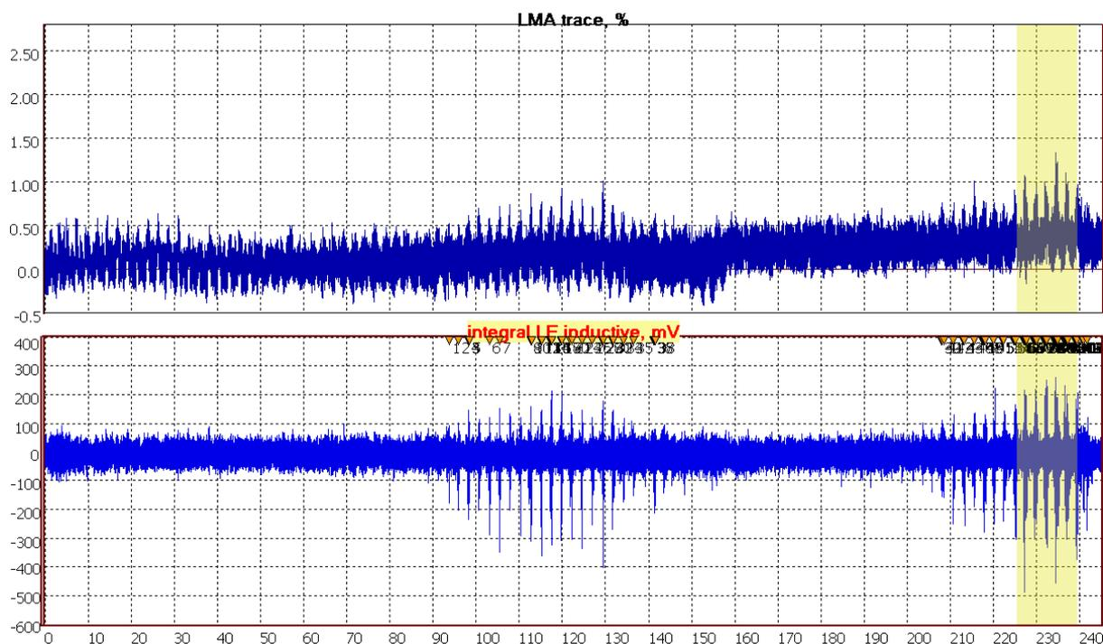
**Figure 5.** LMA and LF traces for the rope running 5400 t-km.
