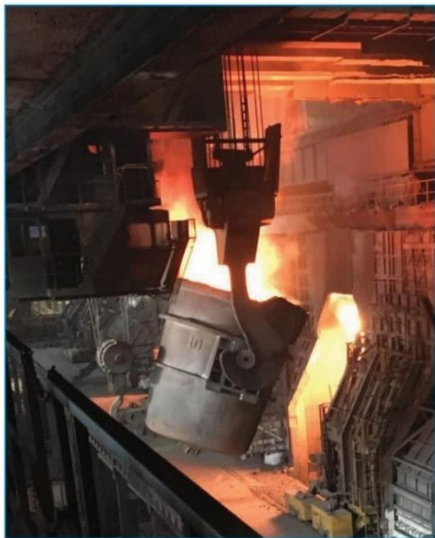
Figure 1. A ladle pouring molten pig iron into a converter.
