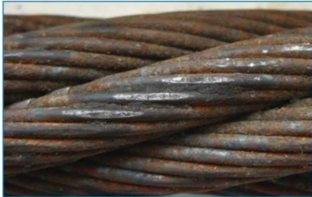
Figure 5. A discarded IWRC rope from a ladle crane ( D = 42 mm, construction: 6 \times 25[1 + 6; 6 + 12] + 7 \times 7[1 + 6] ).
